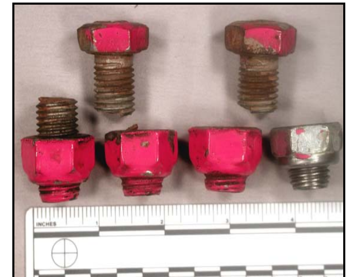
Failed High-Strength Fasteners. How did they fail, and who is to blame? The manufacturer, installer, or the user!
